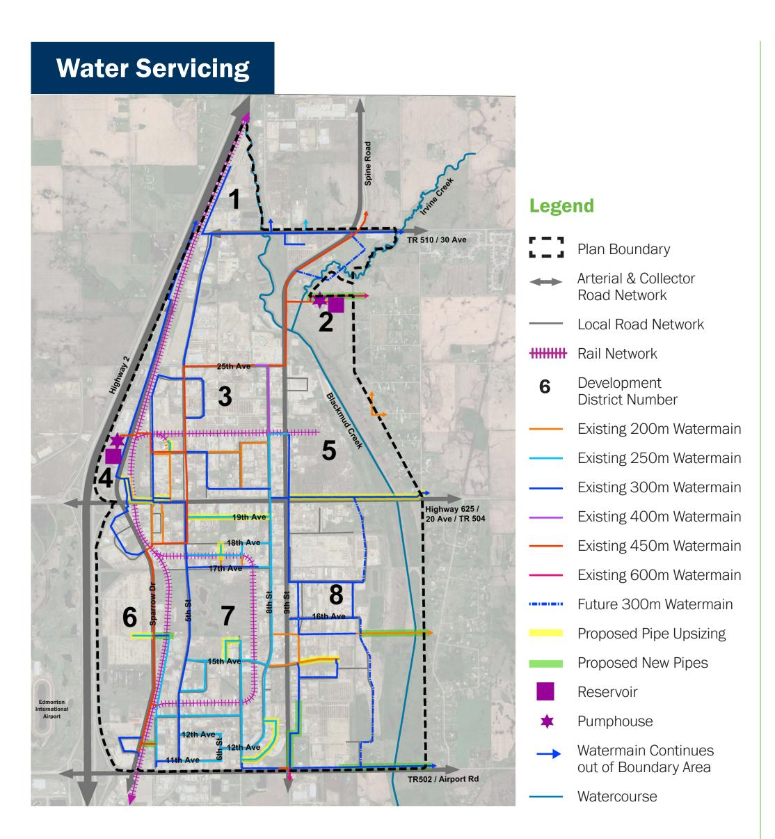
There are 2 pumphouses in the plan area, however the limiting factor for growth are fire flows. To support development, a combination of watermain upgrades and new pipes to complete system loops. Current pumphouses are adequate and will accommodate all future forecasted growth.
