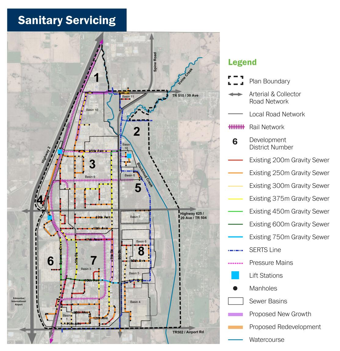
There are has three sanitary sewer lift stations in Nisku. Existing sewers will require upgrades to increase capacity and improve overall system performance.
